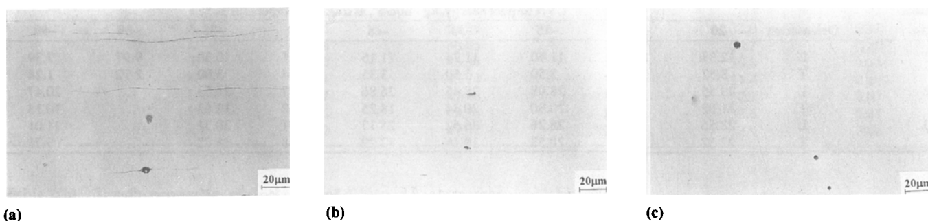
Fig. 2 Optical micrographs of typical inclusions in different steel plates. (a) Heat 1. (b) Heat 2. (c) Heat 3
